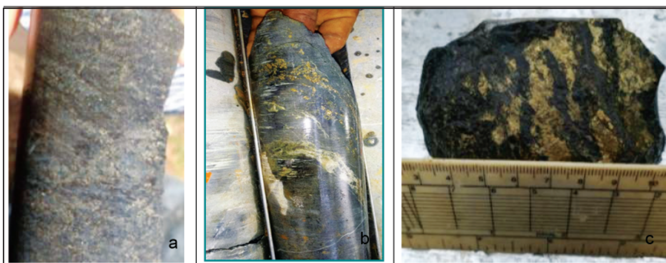
Fig. 8: Chalcopyrite, pyrite occurs as a. Dusty dissemination b. Stringers c. Fracture-filling; Basemetal prospects of Deogarh district, Odisha. (Courtesy: Soumya Ranjan Mishra, Director, GSI, Hyderabad)
