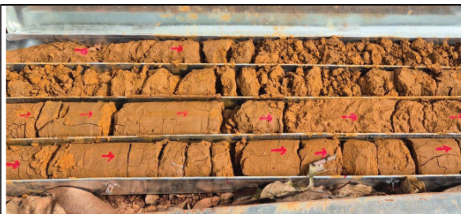
Fig. 12a: Nickeliferous Limonite samples of Kansa Area, Jajpur district, Odisha (Courtesy: Sourav Misra and Dev Lalatendu, Geologist's, GSI, Bhubaneswar)
