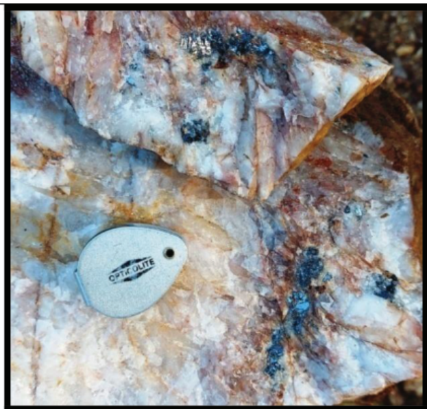
Fig. 9a: Brecciated quartz vein showing streaks of galena near Dumermunda area, Sundargarh district, Odisha (Courtesy: Swanand Govind Pathak)
