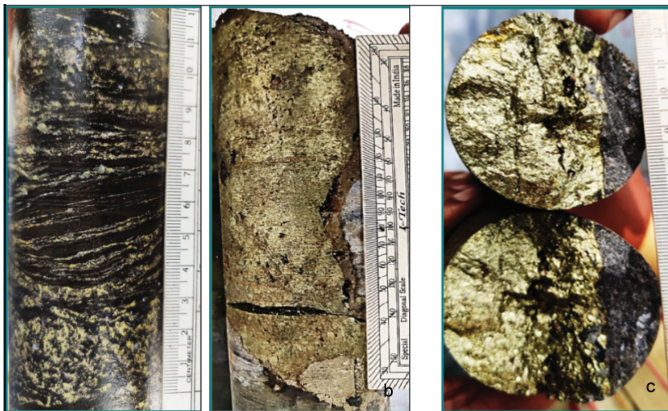
Fig. 7: Chalcopyrite, pyrite occurs as a. stringers b. fracture-filling c. semi-massive; Basemetal prospects of Mayurbhanj district, Odisha. (Courtesy: Harman Mahanta, Sr. Geologist, GSI, Bhubaneswar)
