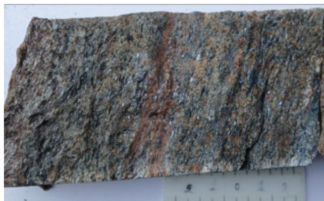
Fig. 11b: Core sample showing graphite of EGMB, Mindol area, Angul district (Courtesy: Itishree Chinnara and Manashree, Sr. Geologist, GSI, Bhubaneswar)
