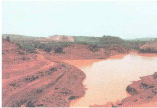
Fig 2.Pits flooded with water: Cause of pit slope problems, Goa
