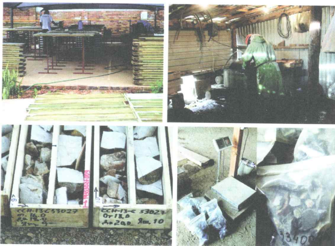
Fig-7: Drill core logging and sampling at Hutti and Charat
