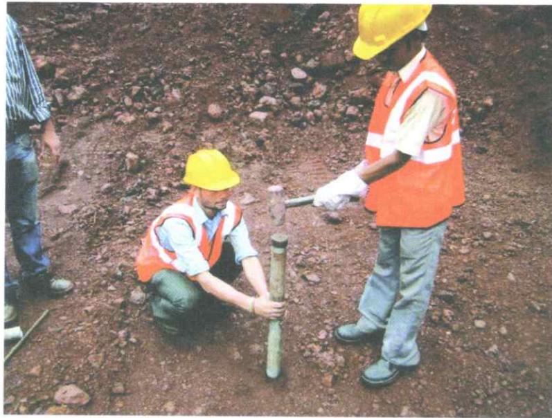
Fig-4: Geochemical sampling using Hand Auger
