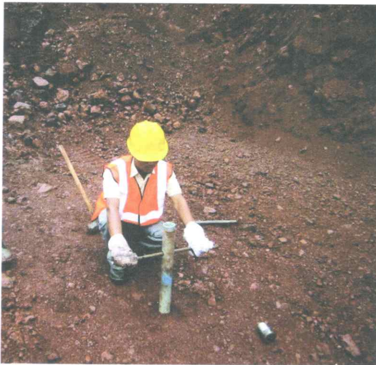
Fig-5: Geochemical sampling collection using Hand auger (b) photo of sample at right after recovery from auger
