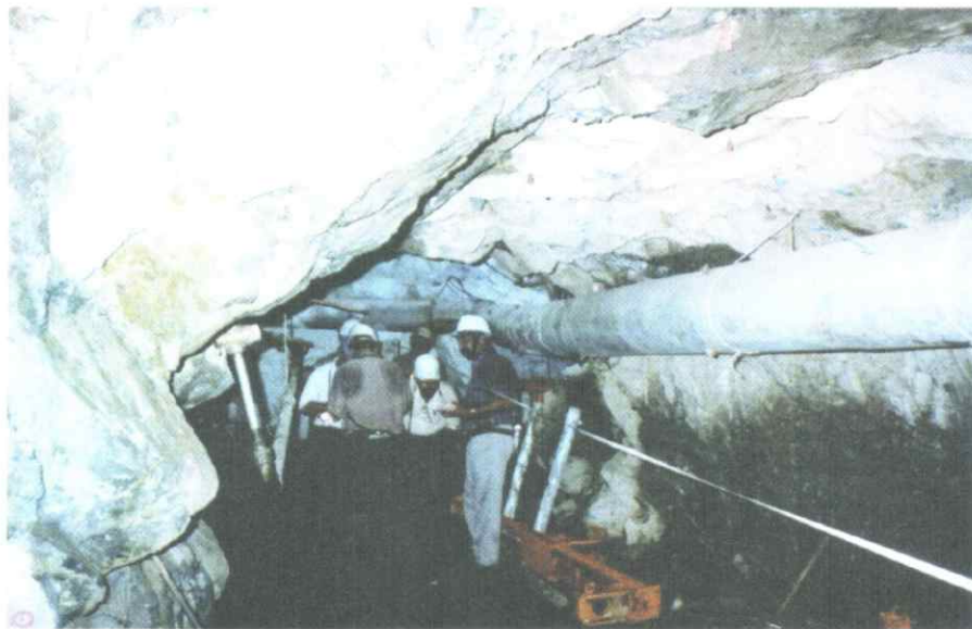
Fig.3. Scan line surveys for mapping joints in underground.
