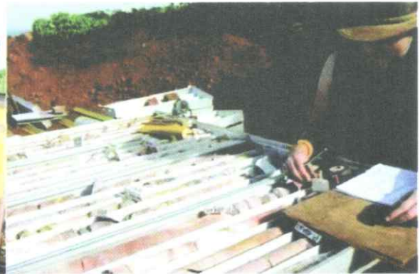
Fig.2. Measurement of RQD from drill cores
